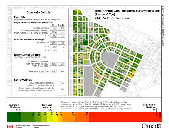
Figure 2: Average GHG emissions (based on modelled energy use) at the level of the housing unit, attributed to the parcel, in the Crescents neighbourhood, Prince George, BC. Spatial Community Energy Carbon and Cost Characterization (SCEC3) model.
